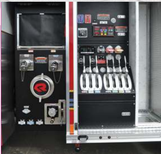
MP3™ Pump Control Panel with Sealed Bank
