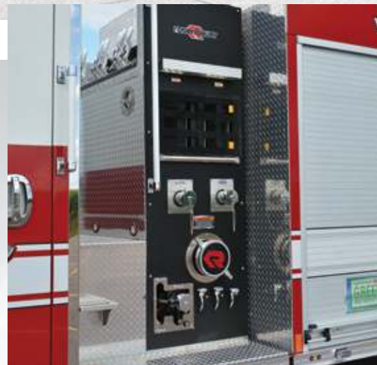
TP3™ Pump Control Panel with Sealed Bank
