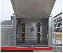
SCBA brackets, SCBA seat backs with lock-n-load brackets
