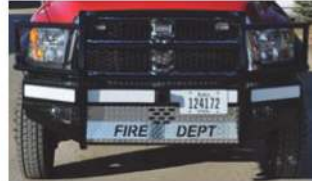
Front bumper configurations with grille guard, TFT Tornado front bumper monitor, warn winch, custom diamondplate, and more
