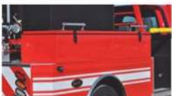
Full depth rear under body storage for backboards, hard suction hose, etc. G3 Fire® poly full length storage trays
