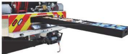
Full depth rear under body storage for backboards, hard suction hose, etc. G3 Fire® poly full length storage trays
